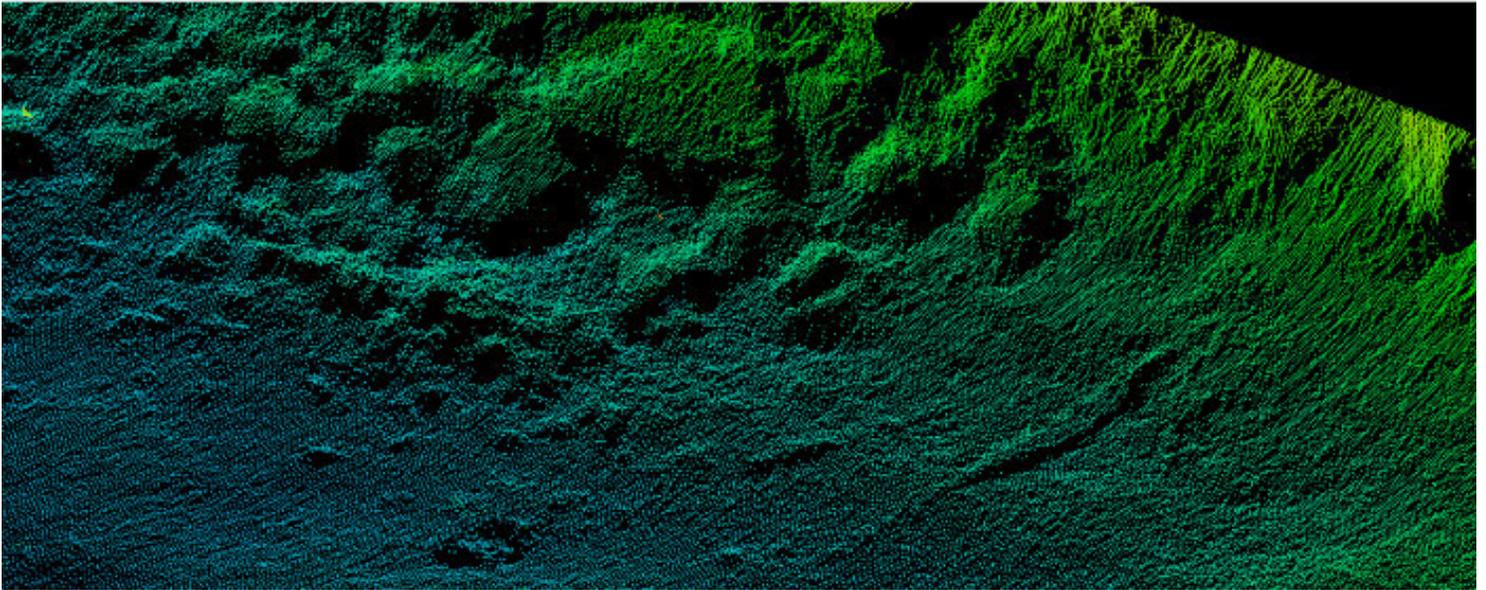
Top: A 600kHz, 100-degree scan from the EM2040. Bottom: A 300kHz scan using the same hardware
